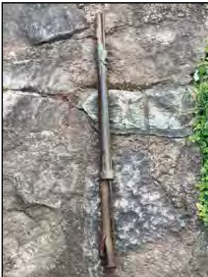
The mystery of this recently-discovered Civil War-era rifle includes what may have happened to cause the barrel to explode at the stock end. Details on page 5.
